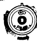
4. To raise the temperature, move black part of knob closer to HI. Each notch equals about 10 F (5 C)
